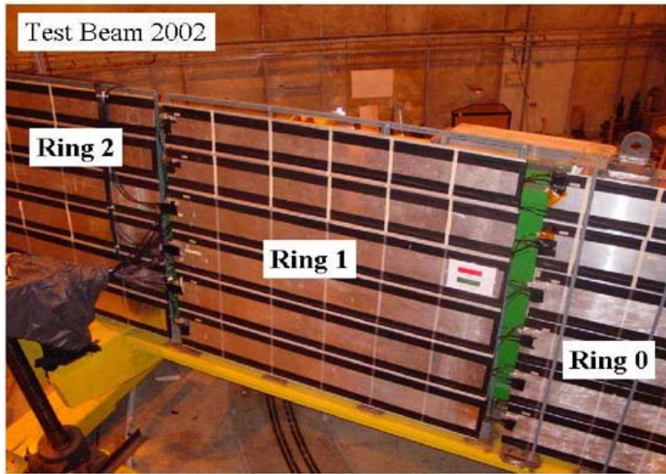
Fig. 4. The Outer Hadronic Calorimeter configuration studied in the 2002 HCAL test beam experiment
