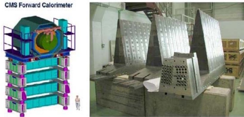
Fig. 6. Left : schematic of the forward hadronic calorimeter (HF). Right : HF modules in construction
